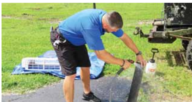
David took all the removable parts outside to be cleaned. The blower wheel was certainly the part needing the most attention
