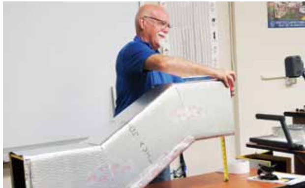
Dave Hilliard of Blacks Supply measures the finished height on his duct transition
