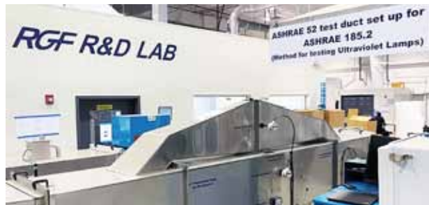
RGF’s expanded R&D Lab & ASHRAE 185.2 Test system
