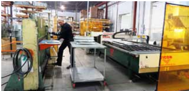
Metal Shop employee fabricating square to round transitions
