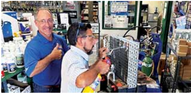
Gil Ledoux of PED Associates instructing proper technique for brazing aluminum
