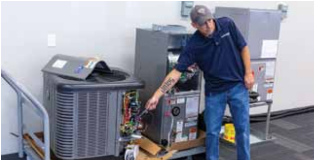
Randy Zolick revealed controls that switch from slow speed inverter control to line voltage for 100% capacity of the new rotary compressors
