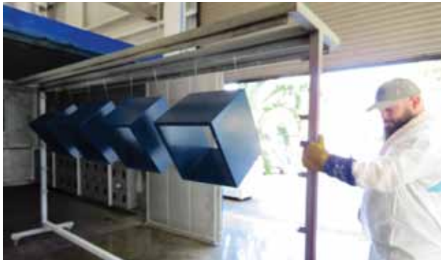
RGF product components that were baked in a special oven after the powder coating process
