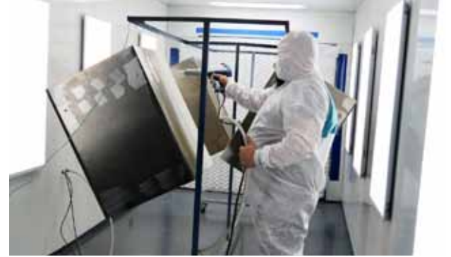
RGF product components that are in the powder coating application process
