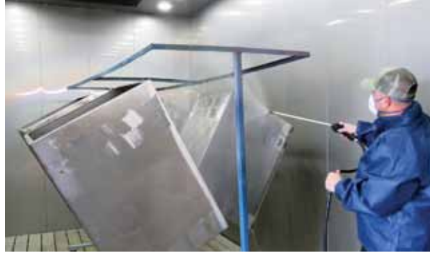
RGF product components being rinsed and pre-treated before powder coating
