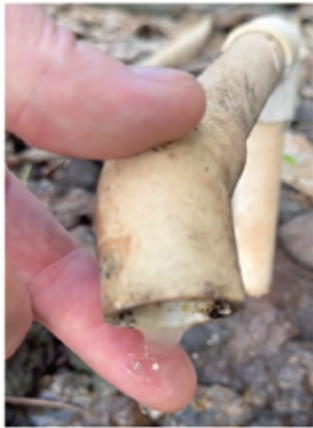
HVAC condensate completely laden with Zoogloea
